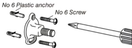
3\_Affix the support to the wall using the screws and the plastic anchors provided. Repeat the procedure (1 and 2) to complete the fixation of the support.
