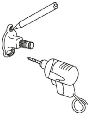
1\_Using the support (in the position the figure shows), mark the place where you will drill the first hole to mount the accessory.
