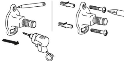
c Mark the places where you will drill before affixing it to the wall using the screws and plastic anchors provided
