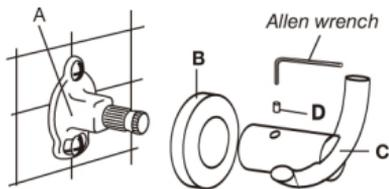
4\_Slide the escutcheon (B) and the main part (C) over the support (A) until it bottom against the wall. Tighten the set-screw (D) with the Allen wrench.
