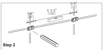
Position the backing plate flat side down on the wall and mark holes with pencil.
