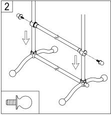
2. Slide middle bar down vertical side bars and tighten bolts at desired evel.
