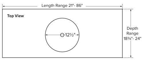
**NOTE:** Counter-sinks with a length of 36" and under have a maximum depth of 23".
