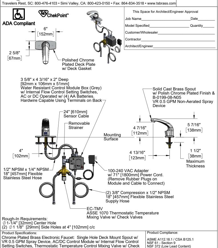
Valves, 18" Flixible Stainless Steel Supply Hoses & 4" c/c Deck Plate
